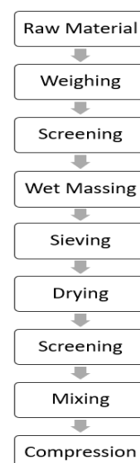
Fig 3. Processing Steps in Wet Granulation
