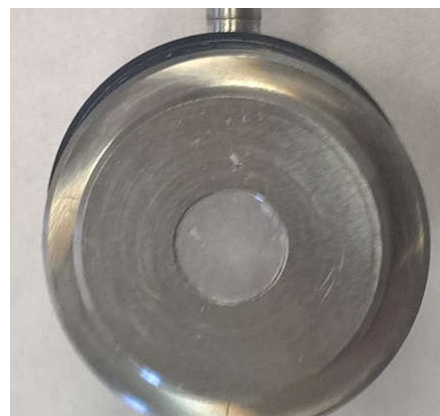
Figure 6. KBr's pellet (example of translucent disk)
