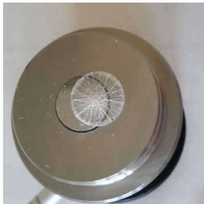
Figure 4. KBr's pellet (example of disk flaking)
