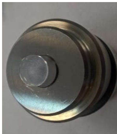
Figure 7. Chrysothile's pellet (example of good distributions and transparencies)
