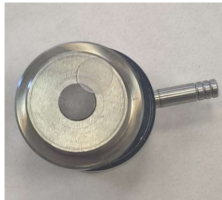
Figure 5. KBr's pellet (example of transparent disk)
