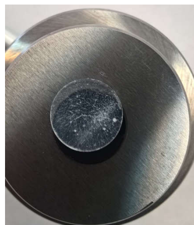
Figure 3. Chrysotile's pellet (example of imperfections and inhomogeneous distributions)
