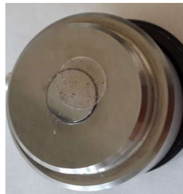
Figure 2. Tremolite's pellet (example of perfect pellet)
